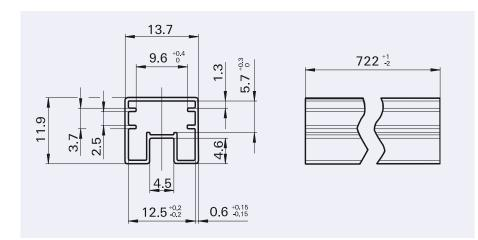
Tube for THT version 50 relays per stick 1000 relays per box
